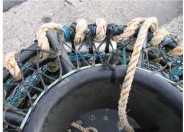
Picture 1b: Temperature-depth sensor fixed in a pot
