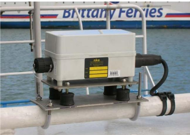
Picture 4: "Concentrator" of data onboard
