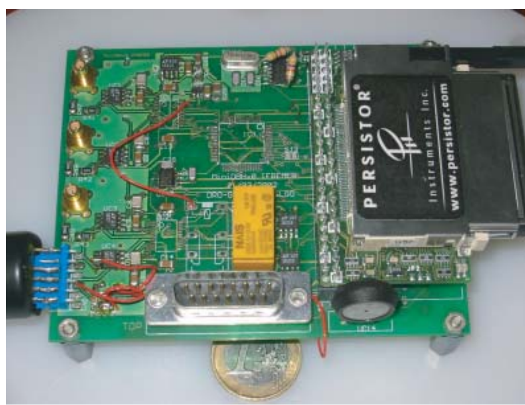
Figure 5 : MicrOBS Electronic printed circuit board prototype for data acquisition and release. Scale given by the 1 Euro coin.
