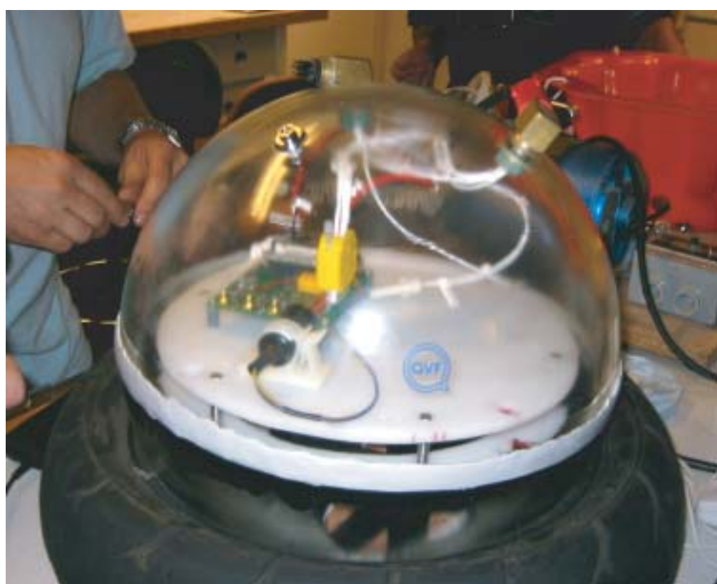
Figure 4 : MicrOBS prototype during sea trials
