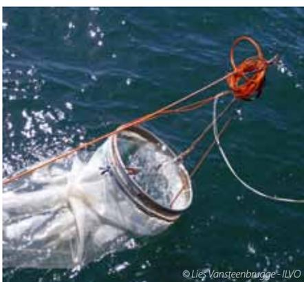
» Sampling is carried out using a WP3 plankton net (net diameter 1m, mesh size 1mm).
