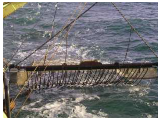
Pulse beam trawl
