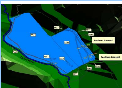
Figures: WEDSS input layer (left) showing wetland hydrogeomorphic units (HGMUs) to be assessed (blue areas) and output layer (right) showing degree of denitrification occurring in HGMUs (denitrification is an important process improving or maintaining water quality and has higher rates in darker areas).
