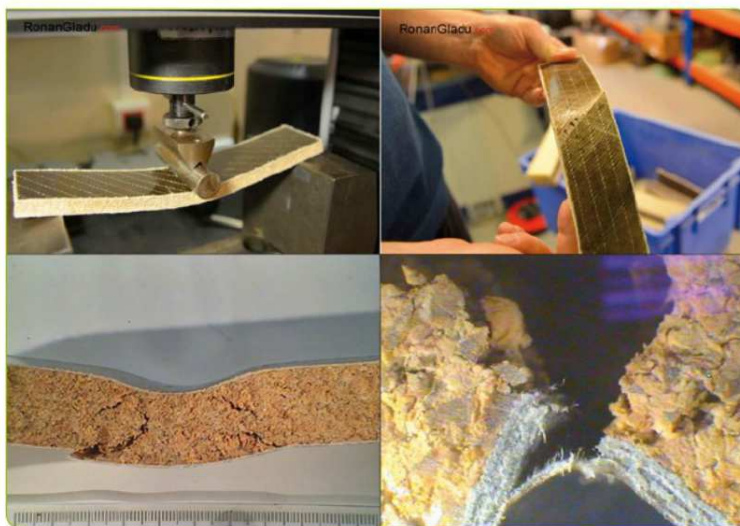
Fig. 2. Evaluation of bio-sandwich materials by extensive testing – here, flax fibre-reinforced facings on cork cores, showing different failure mechanisms (Photos: R. Gladu)
