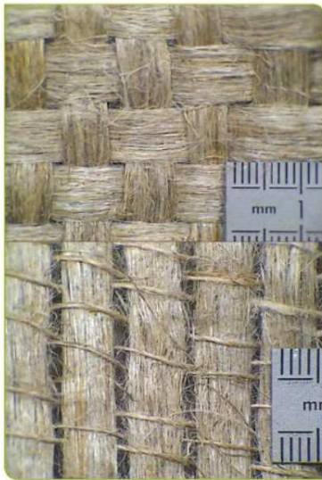
Fig. 1. Flax fibres tested in mat, woven and unidirectional reinforcement forms
