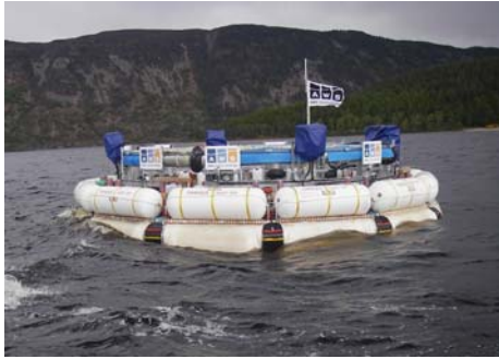
Prototype AWS-III échelle 1/10° - Loch Ness
