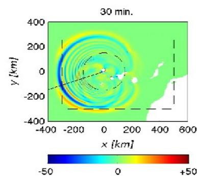
Fig. 5 : Example of tsunami propagation results obtained with Boussinesq model FUNWAVE-TVD for the 80 km<sup>3</sup> case. Dashed black lines indicate the boundary of the sponge layer in the model grid and the size of the initial THETIS grid. Solid black line indicates location of transect of Fig. 4.
