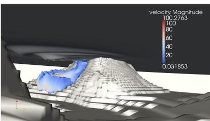
Fig. 3 : Navier-Stokes simulation; results at t=4min for the 80 km<sup>3</sup> case. Underwater view.
