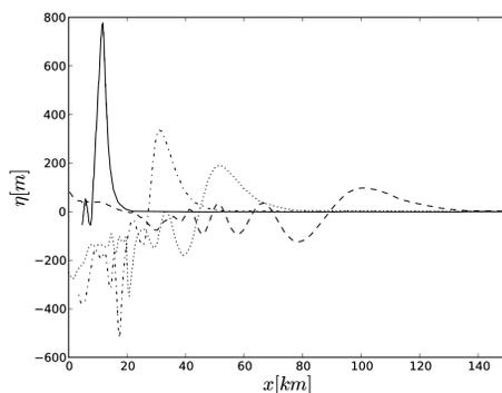
Fig. 4 : Free surface elevation in a vertical plane 20° anti-clockwise with respect to West (see Fig. 5), at t = (solid line) 101 s; (dash-dotted line) 232 s; (dotted line) 340 s; (dashed line) 558 s.
